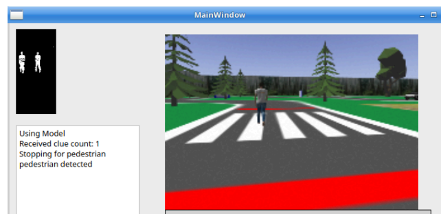
Figure 13. Pedestrian Detection View in GUI (Movement Mask Top Left)
